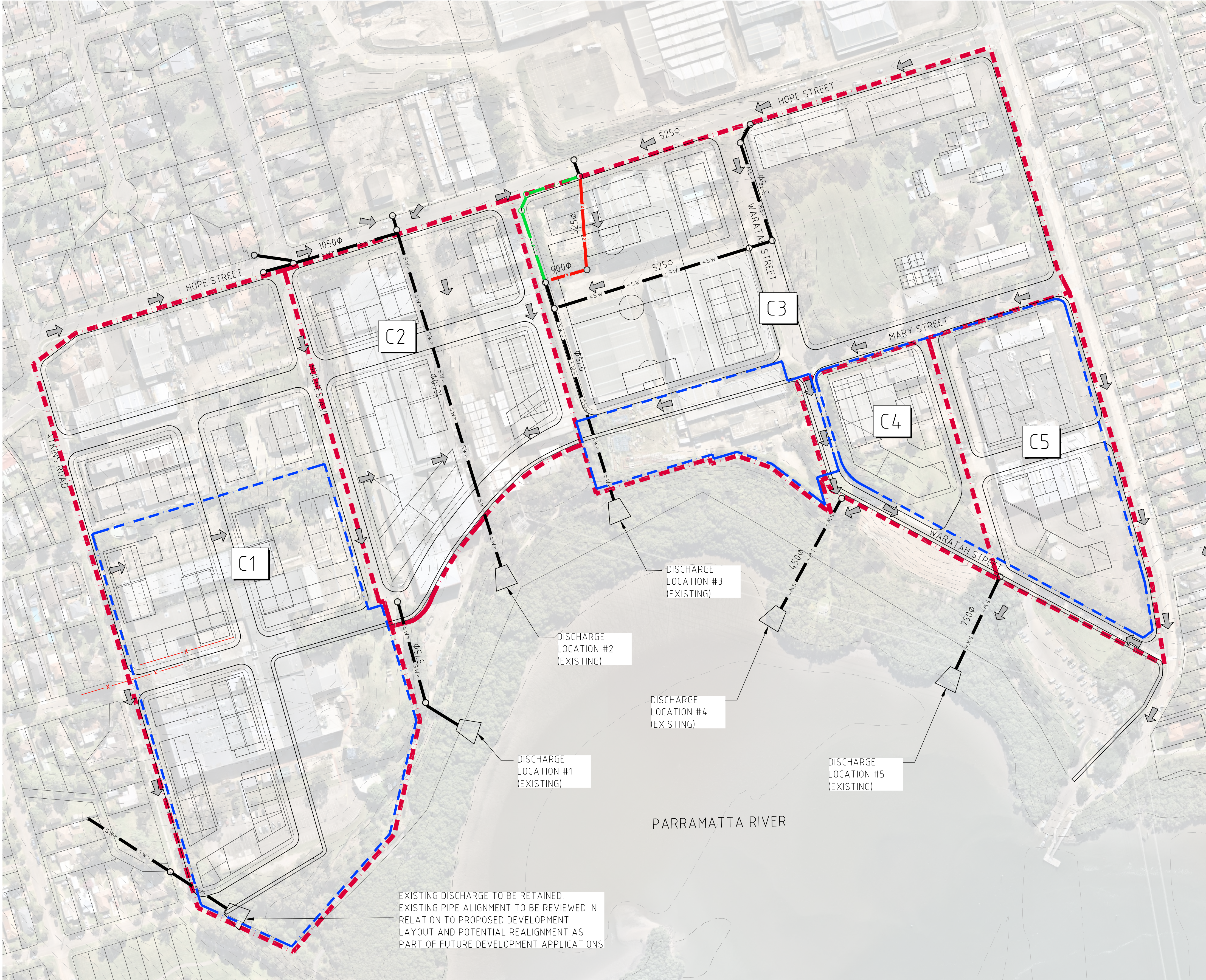
PLAN SHOWING INDICATIVE STORMWATER CONCEPT APPROXIMATELY 1:1500
